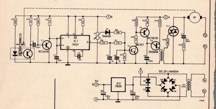
desired and actual motor speeds are compared by T2. T3 and T4 form a trigger pulse generator which produces a pulse to fire the triac once every half cycle of the mains waveform. T2 varies the collector current of T3 and hence the charging current of C6. This in turn controls the point in the cycle
